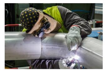
Stainless Steel 316L FC TIG - Coated With Vari-Flow Fluxing System
