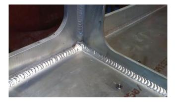
Easy to use – without base metal sagging or wrinkling. Brazing Alloy for all types of Aluminum. Fluxed Residue washes off easily with warm water.
